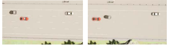
Fig. 5: The diagram of a cut-in scenario in Carla simulator where the red car represents the ego vehicle, with a black car on the left lane attempting to cut in due to the slow-moving white car ahead.
